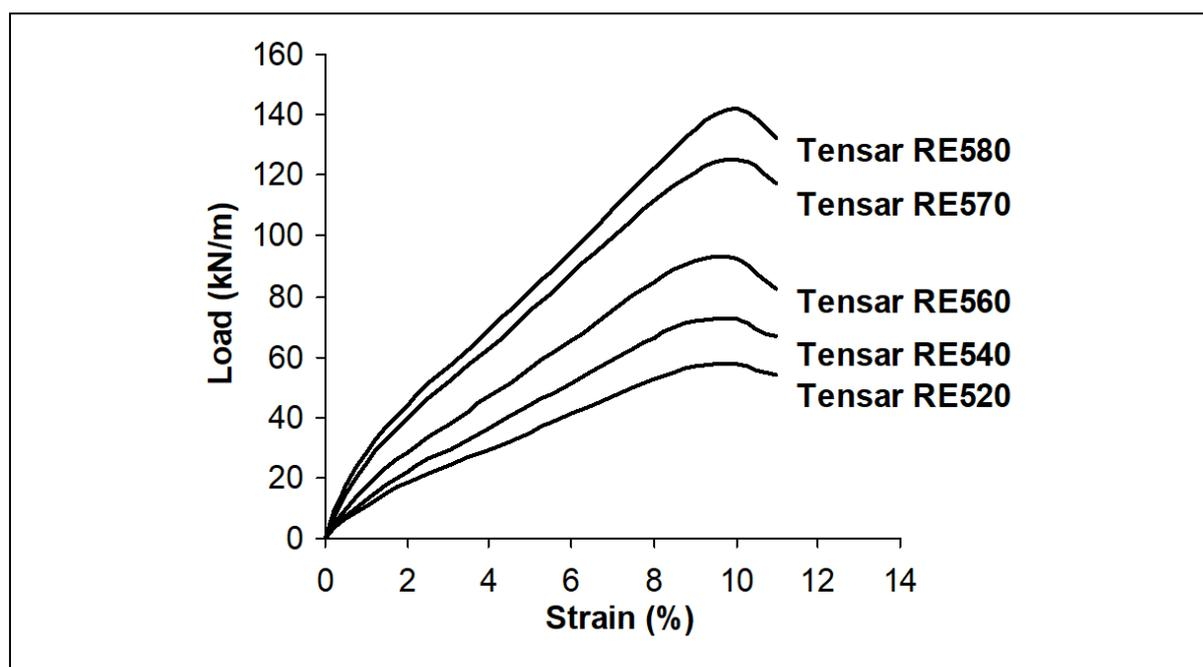
Figure 2 – Typical short-term load-strain properties (longitudinal direction)
