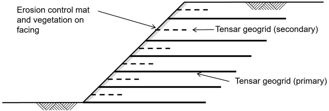
**Erosion control mat protection (slope angle to 45°)**
