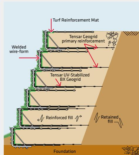
➤ With lower cost materials, reduced labor and the use of lightweight installation equipment, a Tensar® Temporary Wall is the economical alternative.
