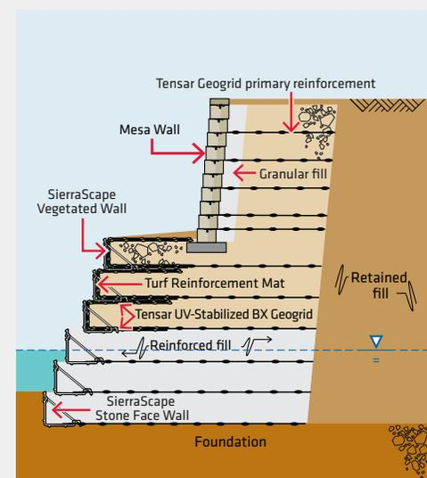
▶ The Sierra® Slope Retention System provides an economical and aesthetic alternative to conventional retaining walls.
