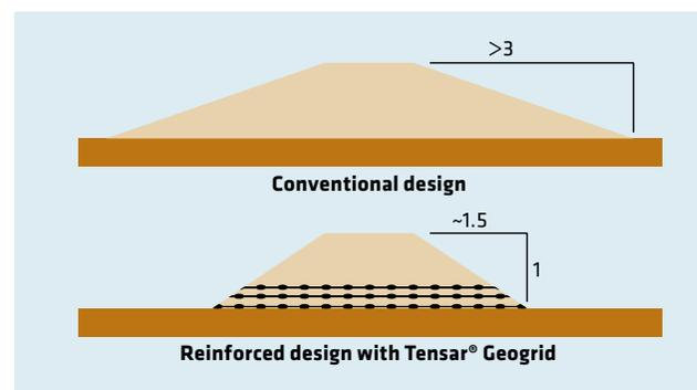
*The Prism System minimizes the "footprint" of the embankment, as well as its fill requirement and settlement potential.*
