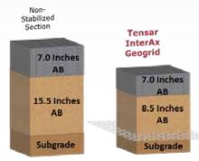
The InterAx-stabilized solution eliminated the need for the additional 7 inches of aggregate that were not in the original design.
