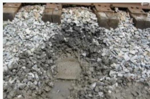
TrackTex exposed, ballast above is wet and free from fines, but the shoulder outside the TrackTex has been recontaminated with mud from the weak subgrade.
