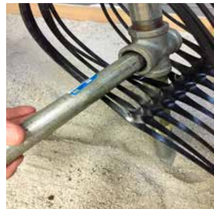
IMAGES M and N: Example of Tensor T-Rod Rake and method for tensioning compound layers of Tensor Geo-Strip.
