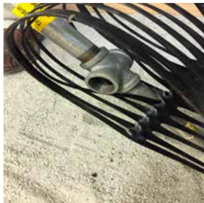
IMAGES M and N: Example of Tensor T-Rod Rake and method for tensioning compound layers of Tensor Geo-Strip.
