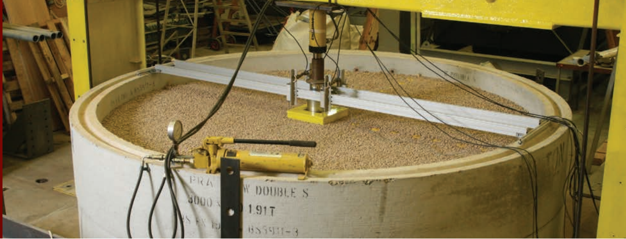
The large 9 foot diameter cylinder at BRE was used to determine the bearing capacity improvement for Tensor TriAx Geogrids.
