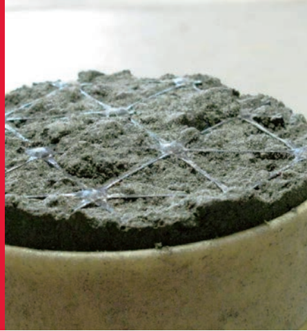
FIGURE 7 Small-scale research through a modified resilient modulus test confirms the stiffness enhancement achieved through the inclusion of a TriAx Geogrid within a crushed aggregate layer.
