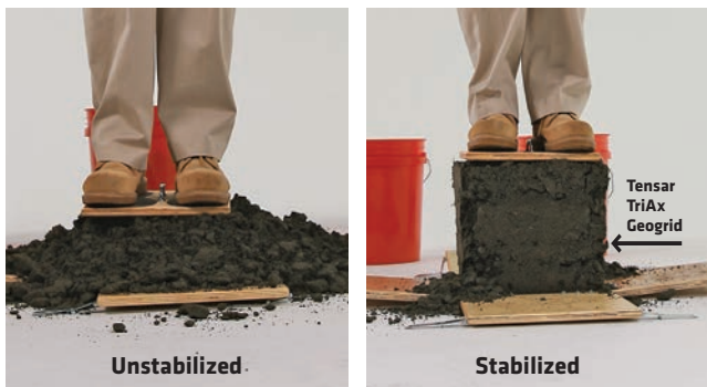
FIGURE 1 The lateral confinement of aggregate reinforcement with Tensor TriAx Geogrid is shown through the box of rocks demonstration.
