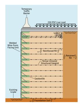
Granite Construction Company contacted Tensar to explore the idea of creating a temporary structure to bridge over an existing highway. The temporary bridge structure would enable the contractor to have access between a concrete batch plant and the construction site, eliminating the need for construction vehicles to enter the highway. Tensar designed temporary walls to support the temporary bridge abutment as well as wing walls for the project with heights upwards of 27 ft.
