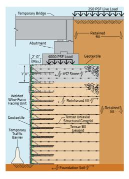
Northeast Remsco worked with Tensar and Kennedy Companies to design and supply the temporary walls for their project. Temporary walls were indicated in the contract documents but Northeast Remsco opted to use the Tensar® Temporary Wall System to act as piers for the temporary bridge structure at multiple bridge overpasses as well. These temporary piers supported a 4,000 psf surcharge load and were designed and installed as four-sided boxes.
