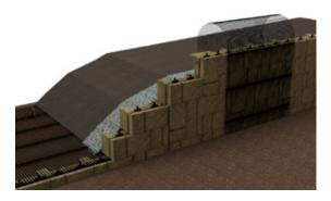
Typically, loose lifts of the reinforced fill shall not exceed 6 in. where hand-operated compaction equipment is used or 10 in. where heavy compaction equipment is used. These thicknesses may vary depending on the approved project-specific soil types used. Compact fill to a minimum of 95% of the maximum dry density, or in accordance with ASTM D-698 (Standard Effort Proctor Test).
