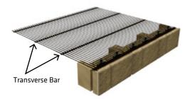
**Step 4 continued:** Snug the geogrid against the connector teeth, and then drive the connector the rest of the way using a rubber mallet.
