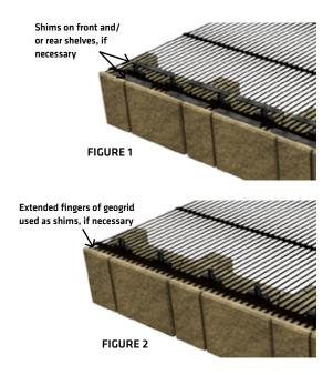
For courses placed on a geogrid elevation, shims may be required on the front or rear shelf of the Olympia Unit (Figure 1 above). The shims should be the same thickness of the geogrid rib. The shim material can be a rib trimmed from the same roll of Tensar<sup>®</sup> Geogrid that is placed on top of the shelf of the unit. An alternative is to cut the geogrid so that the ribs extend approximately 1 in. onto the front or rear shelf (Figure 2 above).
