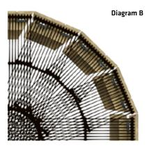
**NOTE:** On tight curves, Tensar Geogrid may be cut lengthwise to the width of the Olympia Units to ensure the transverse bar engages both connectors. The wall designer should consider eliminating the requirement for fill between overlapping layers in areas with a tight radius and/or staggering the layout of adjacent sections of geogrid. From structural walls to tiered gardens and curved walls to stairs, Olympia<sup>®</sup> Walls blend seamlessly with the natural surroundings of any site.
