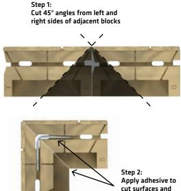
Apply adhesive to cut surfaces and place a #3 rebar bent to a 90° angle into the connection slot
