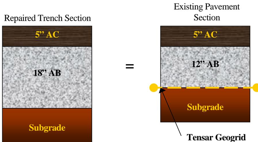
Figure 4 – If proper backfill materials are used and compacted, replacing the geogrid may not be structurally necessary.
