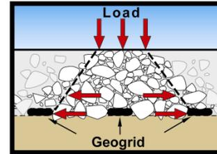
Figure 2 – Stabilization effect of geogrid
