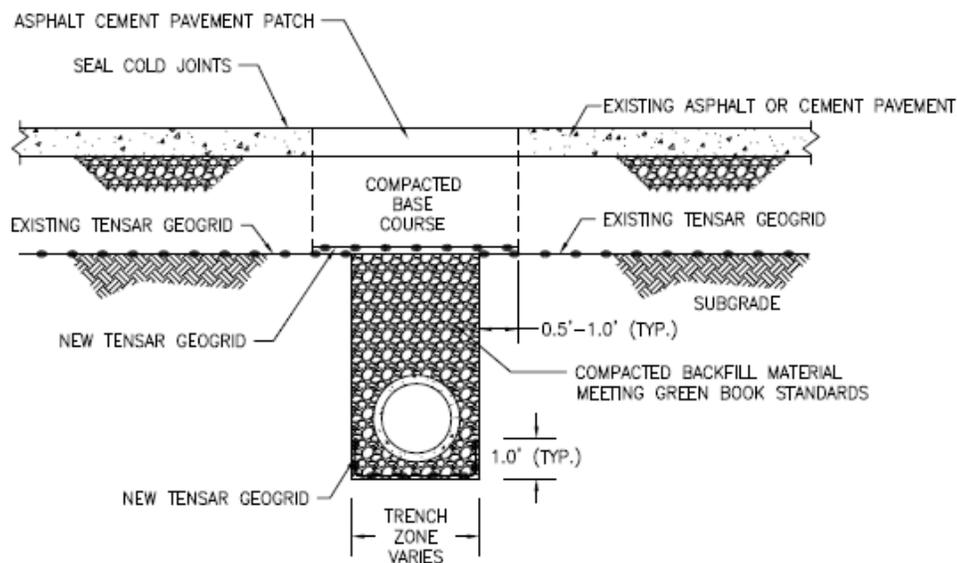
**Figure 5 – Typical Utility Trench Repair Detail (Stabilized Pavement Section)**
