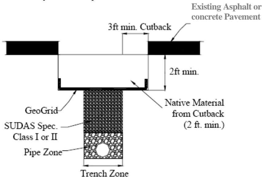
Figure 6 – Proposed cutback and grid placement guidelines. (Source: SUDAS Study, Figure 93)
