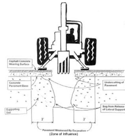
**Figure 1- Loss of support caused by trenching (Source SUDAS study, Figure 9)<sup>1</sup>**
