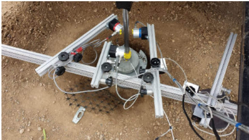
Figure 1: Down-hole confined subgrade test in TX5 section with geogrid pulled back.
