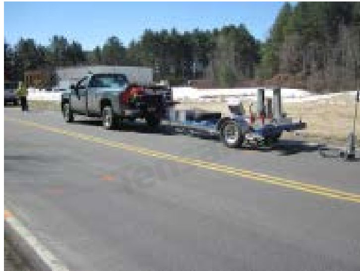
Figure 4: FWD testing performed at four load settings during spring summer and fall. Locations were based on consistent locations
