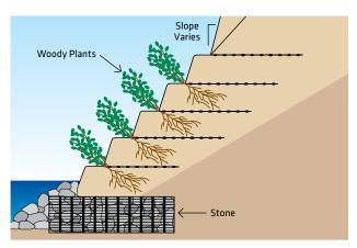
Cross section view of VRSS showing marine mattresses as toe protection and foundation support at the submerged toe of the reinforced slope.
