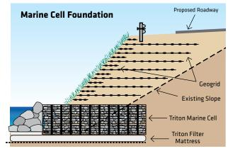
Triton® Marine Cells provide foundations for embankments, MSE slopes or walls and improve not only constructability, but also stability, bearing capacity and distribution of pressure.
